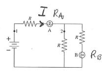
b. Bulb A is replaced. Bulb B is then removed from its socket. What happens to bulb A? Does it get brighter, stay the same, get dimmer, or go out? Explain.
